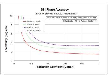
Corrected system performance with 3.5 mm device connector type, N4691B electronic calibration (ECal) module
