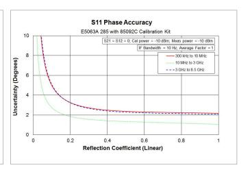
Corrected system performance with 3.5 mm device connector type, 85033E calibration kit
